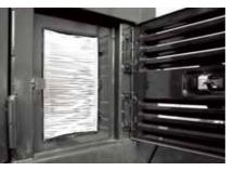
Air Purification Filter It effectively filters dusts out of the cab to keep the air clean and fresh.
