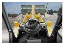
Spacious Cab with Excellent View Spacious cab designed with ergonomics approach boasts low noise and excellent view, arc shaped front window, large rear window and side windows offer wide view in all directions.
